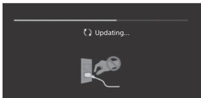
Do not unplug the AC power cord (mains lead) during the software update. If you do, the software update may not finish completely, and it may cause a software malfunction. Software updates can take up to 30 minutes. If you do not wish to update the software automatically, press **HOME** and select [Help] → [System software update] → [Automatic software download] → [Off].
