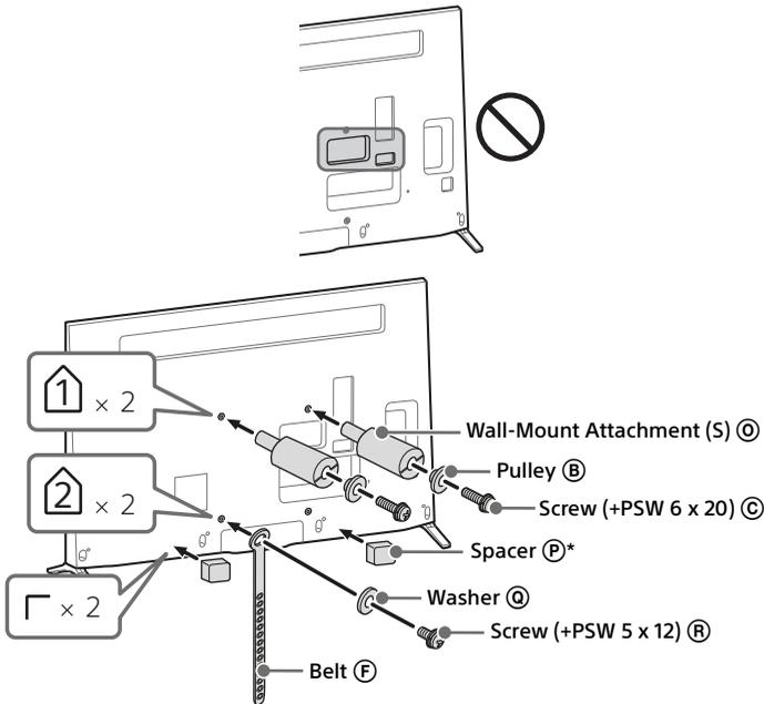
\* Attach Spacer (P) on the flat area indicated by the marking  $\Gamma$  after peeling the separator.
