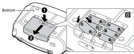
Use alkaline batteries with this unit. The use of manganese batteries is not recommended, since this type of battery has an extremely short usage time.
