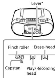
\* Expose the erase-head by pressing the recording button **[5]** while holding down the lever with your finger.
