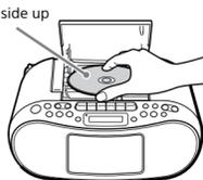
The disc is loaded and the disc information appears on the display. The information displayed varies depending on the disc type (audio CD/MP3 disc).
