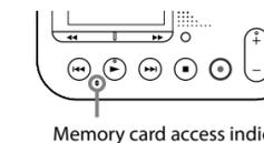
The memory card access indicator is flashing in orange when the memory card recorder is accessing the memory card. Do not remove the SD memory card, batteries, or disconnect the AC adaptor while the memory card access indicator is flashing.
