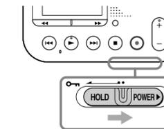
Slide the HOLD-POWER switch in the direction of "POWER" and keep it there until "Power Off" animation appears. The memory card recorder will turn off in a few seconds.
