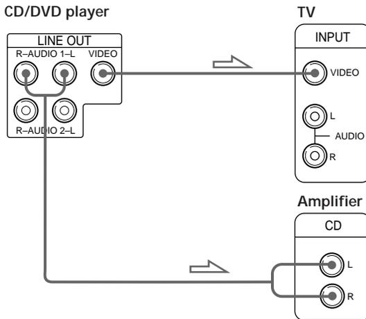
Make the same connections when your amplifier conforms to "Pro Logic."
