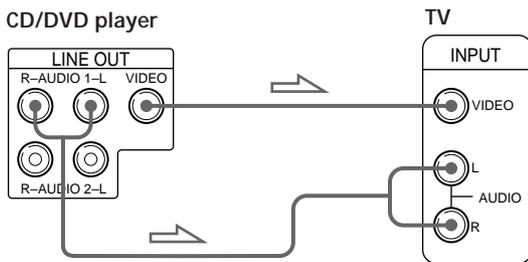
p To listen to the sound through speakers connected to an amplifier
